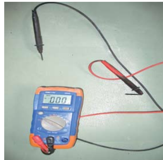
The incorrect meter used by the electrician
