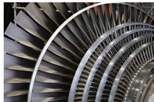
Gas turbine rotor
