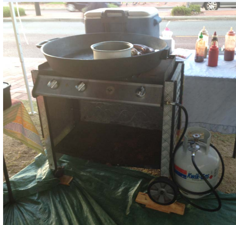
BBQ modified to restrict air flow around burners and plates so that a large pan could fit on burners
